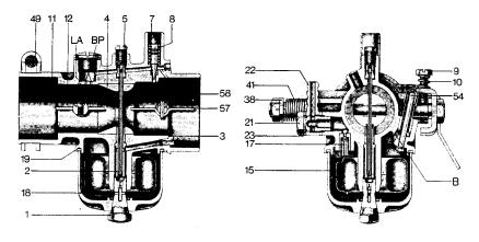
The idling speed quoted for a particular engine serves as a guide only. It may sometimes be necessary to make minor adjustments. First, run the engine until warm and select the desired idling speed by using the idling adjustment screw (9). The mixture control screw is then opened carefully, starting from the basic position, until the engine speed rises. The screw is then closed again by approximately one quarter of a turn.
