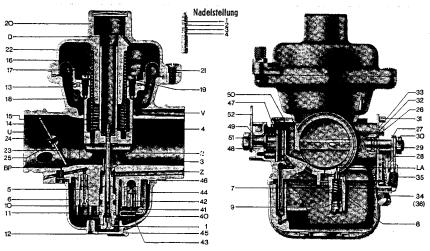
zontal position until the float just contacts the float needle. In this position the pointer on the float hinge is set in such a way that the float top edges are parallel to the top edge of the float chamber.
