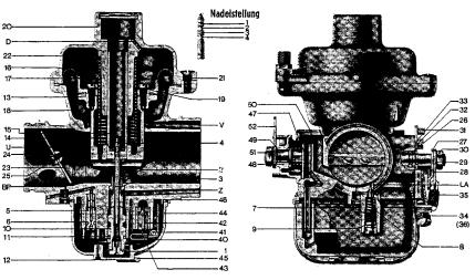
pushed up or down, the retaining spring engaging the next notch in the jet needle. If the needle is suspended higher up, this will result in a richer mixture and vice versa.
