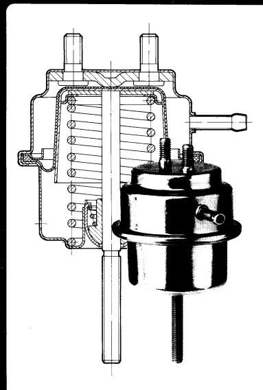
As an air pressure element the BING-Actuator Type 89 is developed to operate under high temperature. Therefore it is well suited for the controlling of supercharging engines (e.g. application in production for waste-gates in COMPREX-pressure-wave superchargers.)
