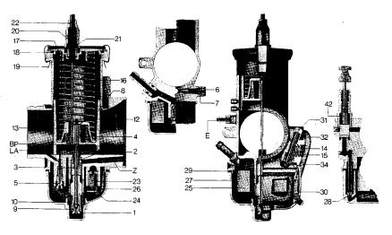
provided by an auxiliary system, the idling system, which consists of the idling jet (5) with the fuel filter (11) and the mixture control screw (6) with sealing ring (7), which acts as a seal for the screw and also stops it from working loose.
