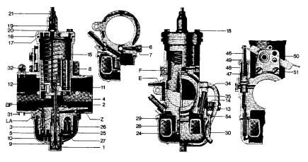
tion 2" means that the jet needle has been suspended from the spring retainer (11) with the second notch from the top. When the throttle slide opening is reduced further, the amount of fuel supplied is affected also by the shape of the throttle slide at the lower end. With increasing height the cylindrical recess called air cushion results in the mixture becoming leaner. The recess on the filter side called cut-out has a similar effect but this extends up to a greater slide stroke.
