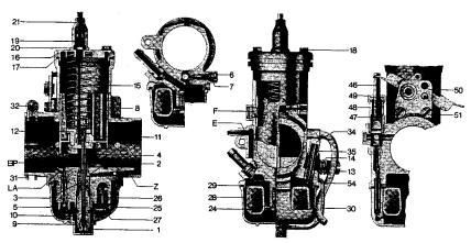
fuel needle spring is not compressed by the float weight. It is therefore advisable to put the carburettor in a horizontal position until the float just contacts the float needle. In this position the pointer on the float hinge is set in such a way that the float top edges are parallel to the top edge of the float chamber.
