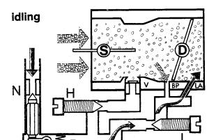
In a special version, the fuel for the idling system can be drawn after the main jet (**H**): dependent idling system. The advantage of this arrangement is that the idling system is less active when full power operation is required; it is regulated by the main jet (**H**) alone.
