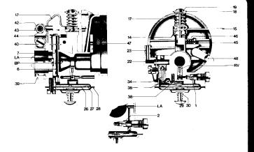
governor rod, or the spring (17) on non-governed engines engages. When operating with a governor, the spring (17) acts on only one side of the throttle lever and serves to close the butterfly valve when idling.
