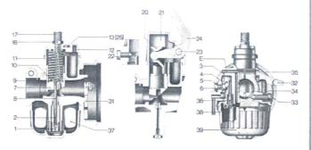
to the jet needle cone, affect the amount of fuel drawn in. For example a higher needle position results in a larger annular cross-section in the needle jet which allows more fuel to pass through and vice versa. "Needle position 2" means that the jet needle has been suspended from the sprung retainer (9) from the second notch from the top.
