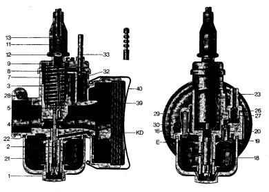
washer (6) so that the jet needle can swing freely during operation. With a small throttle valve opening and in particular during idling, the amount of mixture supplied is affected also by the underside of the throttle valve. It can have the shape of a cylindrical recess, a chamfer on the filter side or a slot leading towards the engine side. A number of differently shaped throttle valves is available for adjusting the carburettor. These are termed "cutaways".
