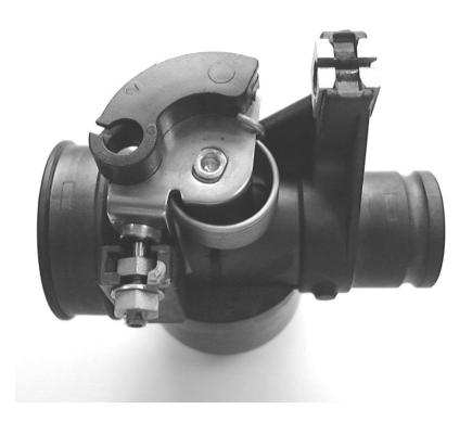
The first serial plastic throttle body for small displacement engines up to 100 cc. It controls and informs about the air flow of an injection system. According the plastic housing, the cable quadrant and the integrated throttle position sensor the throttle body weighs only about 110 g. For safety reasons the position sensor is equipped with double tracks. The cable fixing is adjustable.
